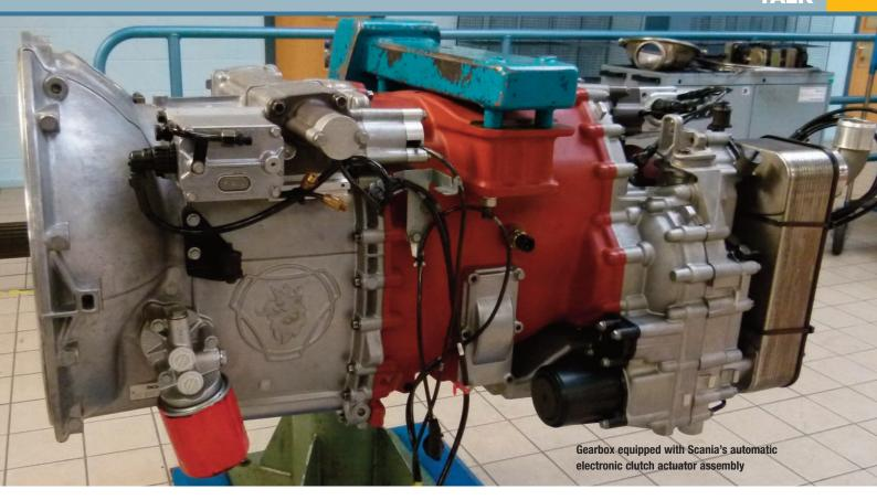
lay shaft dips into the transmission fluid pool and throws oil between the gears for extra lubrication. Low drag gearboxes extend that action to reduce gearbox fluid by two or three litres, and hence reduce frictional losses without compromising lubrication.
