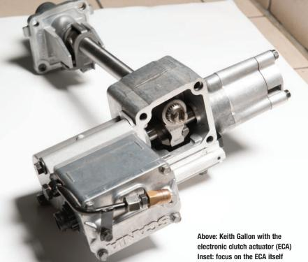
and deliver the required clutch action. That, in turn, increases pressure in the slave cylinder at the requested rate and pops the clutch.
